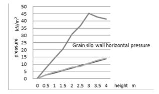
Fig. 2. Pressure exerted on wall of grain silo filled in with wheat. The curve above is Lateral pressure curve of tube wall without pressure reducing tube. The curve below is Lateral pressure curve of tube wall with pressure reducing tube.
